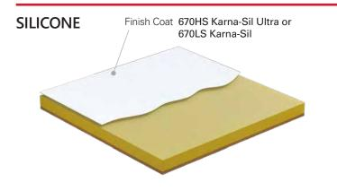
Note: This represents newly-installed spray foam roofs, which do not require cleaner or repair products. For information about systems for previously-coated spray foam roofs, please contact Karnak.
